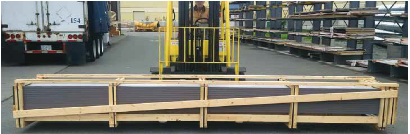
Spread forks evenly under each bundle/lift/skid/crate
