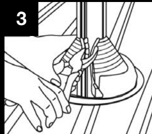
3 Squeeze jointer tightly with pliers, start at the top and work down to the base.
