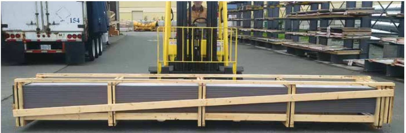
Spread forks evenly under each bundle/lift/skid/crate
